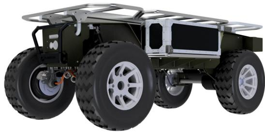
The **HIGHLAND-500** platform is an electric unmanned ground vehicle with excellent maneuverability, a lot of space storage and high precision steering.
